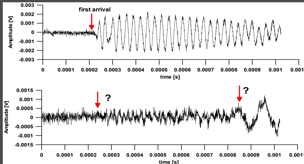
bad signal-noise ratio traces need signal processing technique application for travel time detection and uncertainty determination
