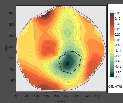
Evolving condition monitoring tested with laboratory measurements of velocity variation maps.
